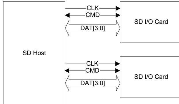
**Figure 2-1 Signal connection to two 4-bit SDIO cards**
