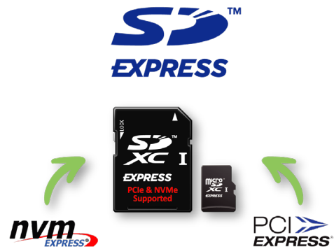
Figure 1 SD Express – A Combination of Three Leading Standards
