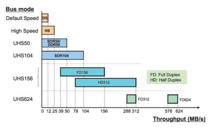
Figure 2: Progress of Bus Interface Throughput
