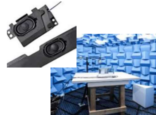
Audio issue, Check in Acoustic chamber
