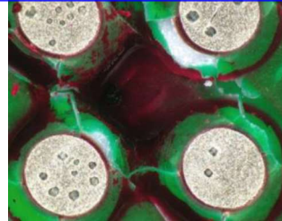
Solder issue, check via Red ink & Microscope
