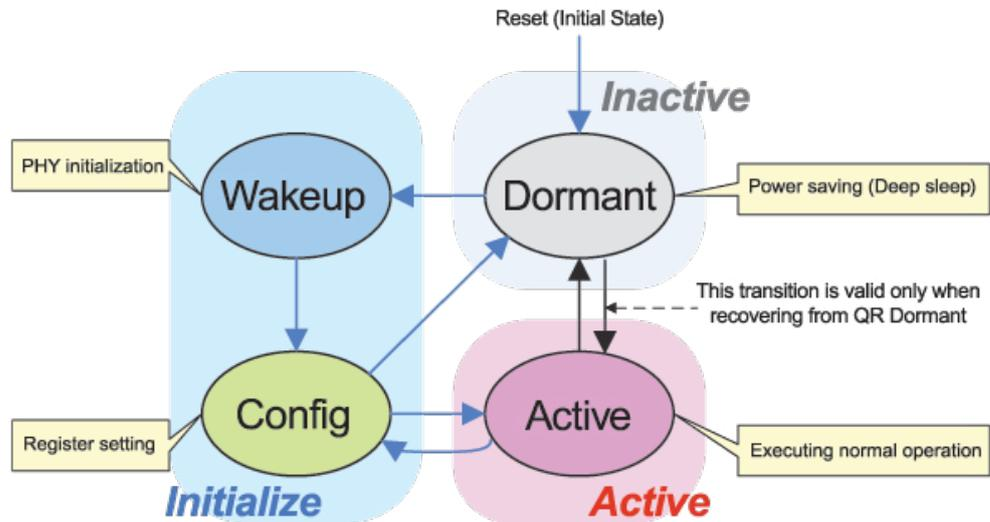
Figure 3: State Machine for UHS-III
