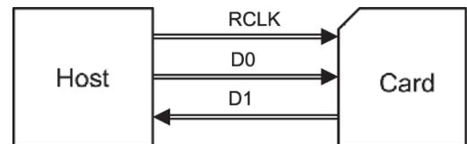
Figure 1: Interface Structure of UHS-III (Full-duplex Mode)
