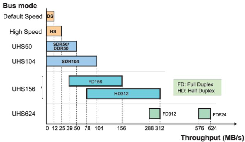
Figure 2: Progress of Bus Interface Throughput
